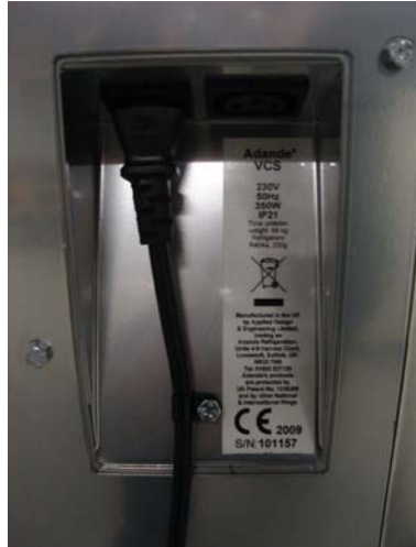
Figure 3a: Mains connection point
