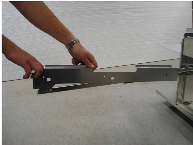
Figure 23: Removal of drawer support from the drawer runner.
