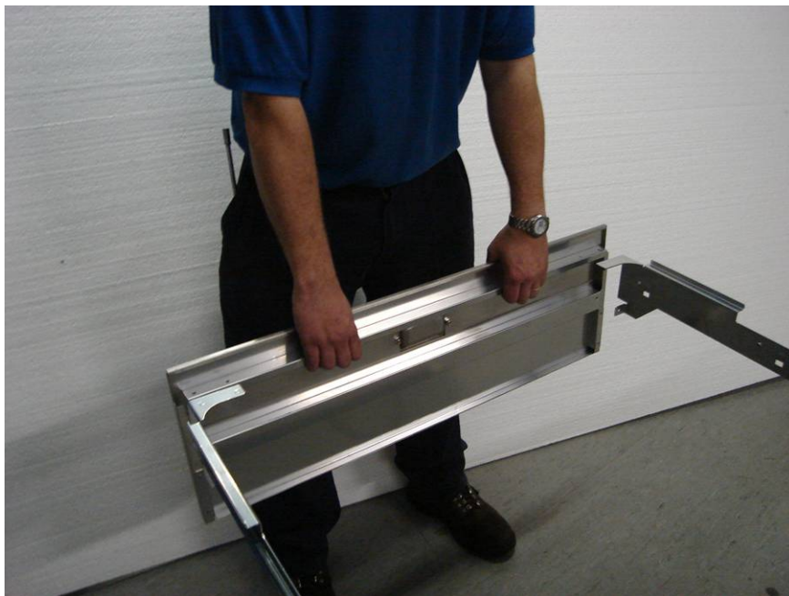
Figure 12: Removing the drawer front
