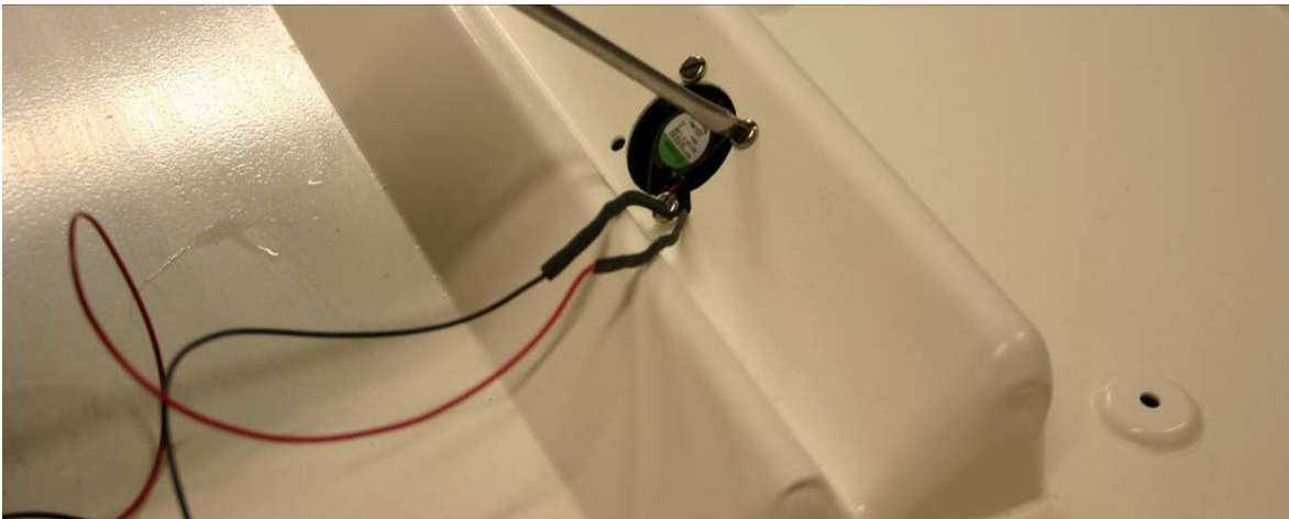
Figure 16a: Evaporator fans
