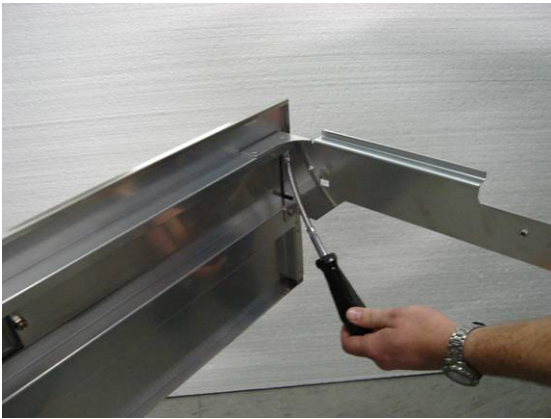
Figure 11: Removing the four bolts and two screws
