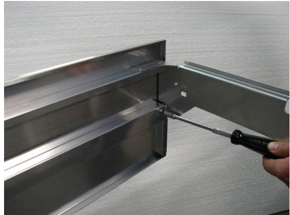
Figure 11: Removing the four bolts and two screws
