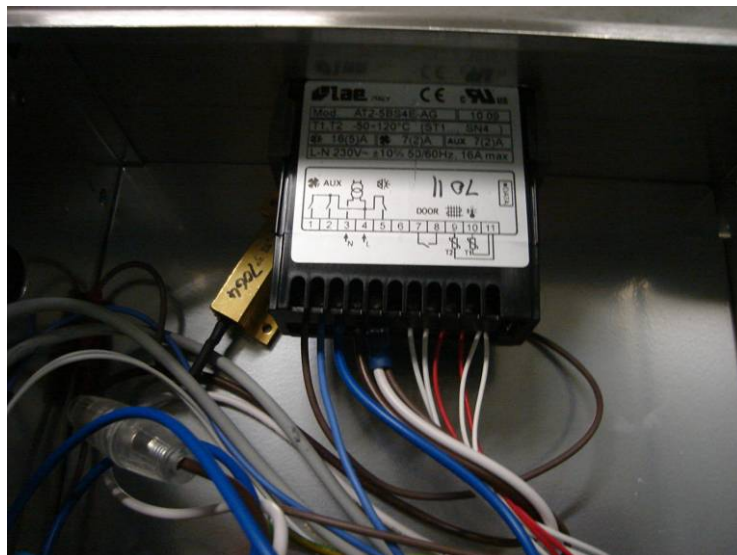
Figure 27: Wiring connections to AT2 controller
