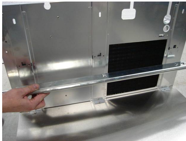
Figure 24c: Fixings in vertical wall supports and lancing in runner outer beam
