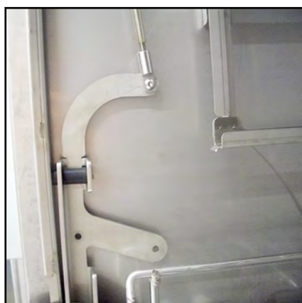
Fig.1: Articulated rod at bottom before the conversion
